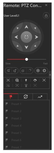
Figure 5-1 PTZ Control Panel
