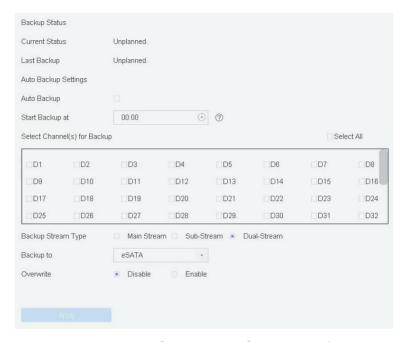
Figure 11-6 Configure eSATA for Auto Backup
