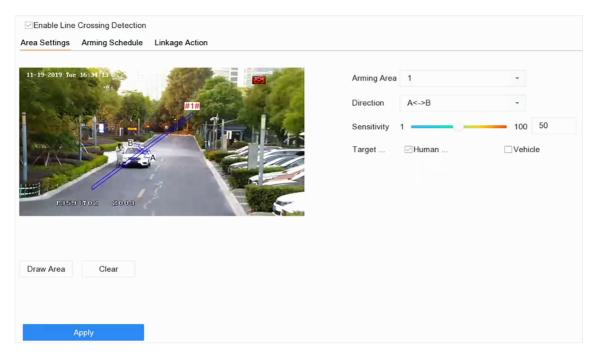
**Figure 6-5 Line Crossing Detection**
