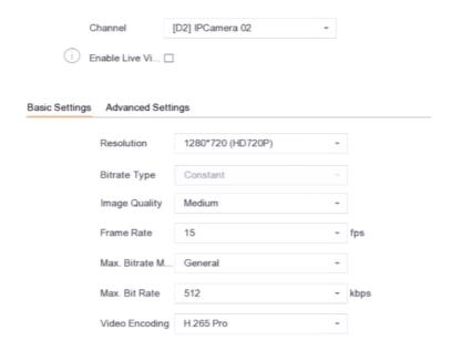
**Figure 3-6 Transcoded Live View**
