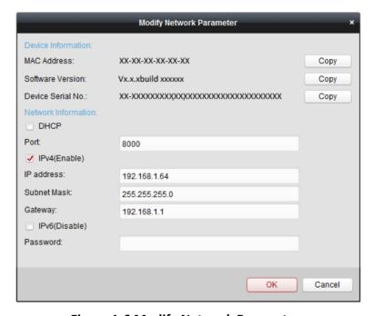
**Figure 1-6 Modify Network Parameters**
