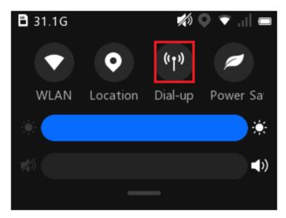
Figure 6-3 Enable Dial-up from Notification Center
