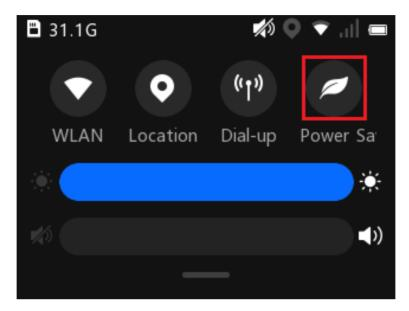
Figure 7-1 Enable Power Saving Mode from Notification Center
