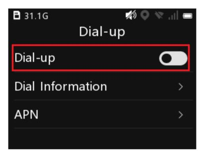
**Figure 6-4 Enable Dial-up from Network Settings**
