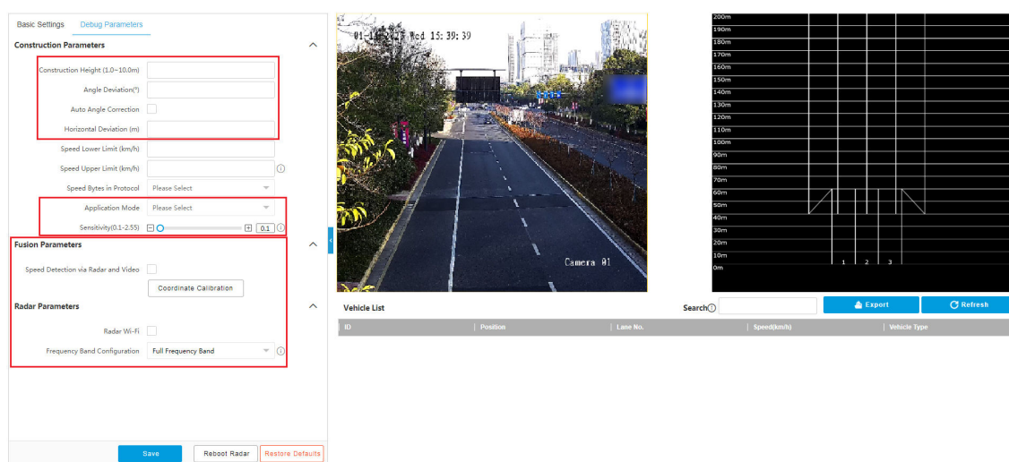
Figure 3-6 Debug Parameters for Speed Detection via Radar and Video
