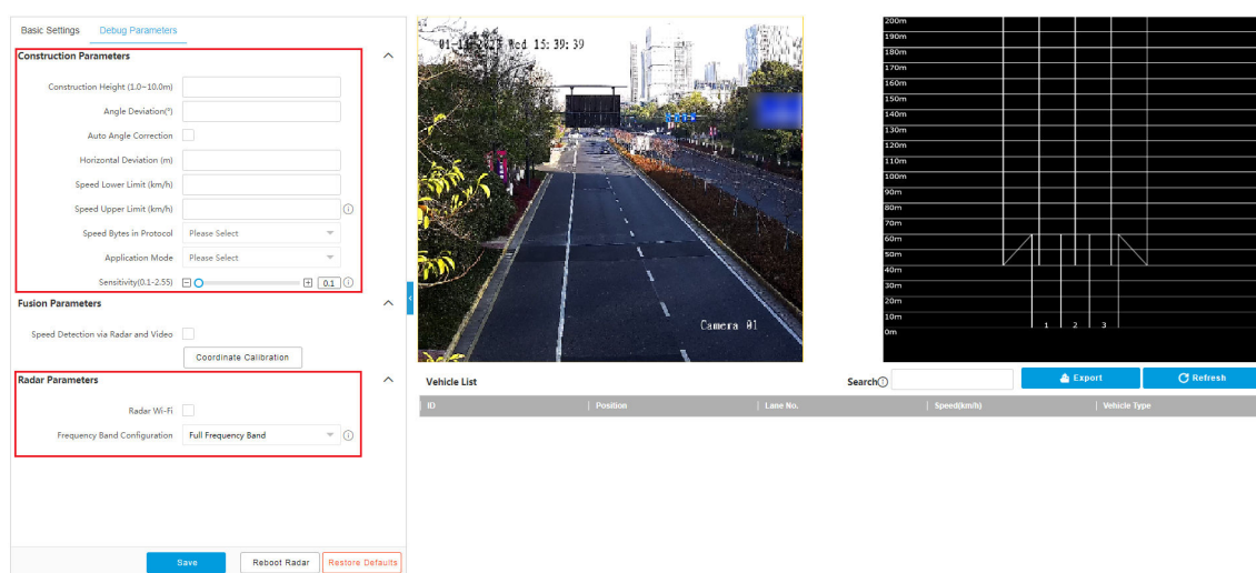
Figure 3-3 Debug Parameters for Speed Detection via Radar
