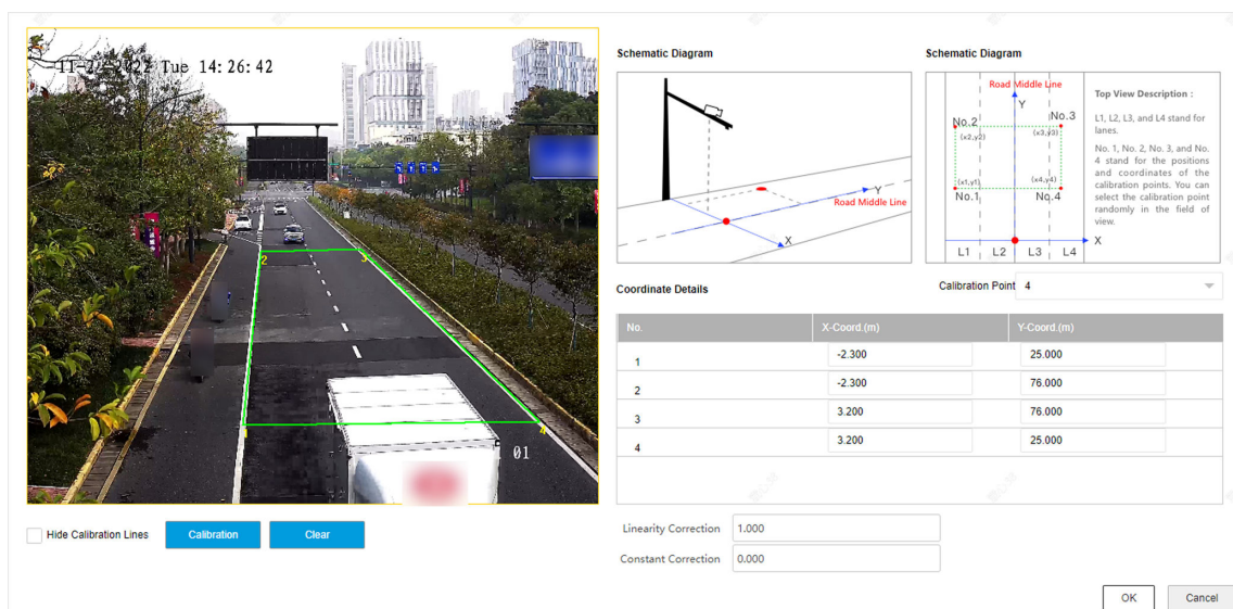
Figure 2-12 Calibrate Speed via Video
