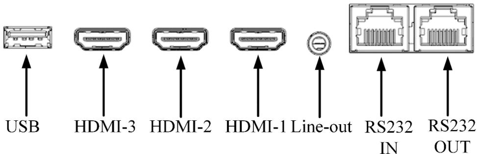
Figure 1-2 Interfaces on the Rear Panel
